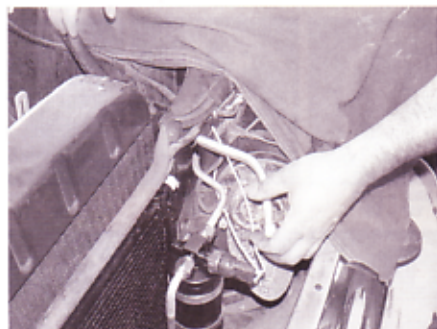
15. For a cleaner look, Manny plumbed the drier and condenser with hand-bent hard-lines instead of the rubber hoses provided.
