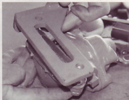
5. A bead of silicone was then applied to the block side of the water pump, a new gasket was fitted, more silicone was applied on top of the gasket and the new bracket. The bracket was then fitted over the bolts, another bead of silicone was applied and another gasket fitted and siliconed.
