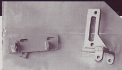
The compressor brackets from Patrick's Antique fit the block perfectly, but one mounting ear on each bracket had to be cut off, repositioned and re-welded. Benny also painted the brackets and spacers gray to match the engine.
